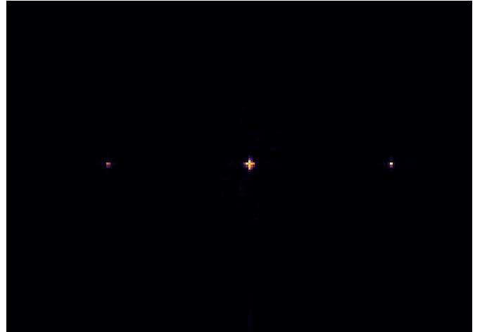
(c) Correlation plane intensity, showing the cross-correlation peaks at the off-axis positions.
